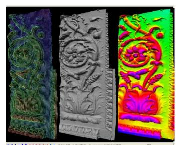
The multi-image matching combines several matching algorithms and works on pairs, triples or entire image blocks. The package has been adapted and modified from the SAT-PP software and has proven its quality and performance in many Cultural Heritage projects.
